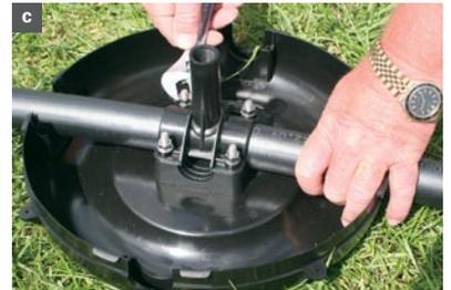
Select the Riser to suit your sprinkler size. Ensure fastening nuts are tightened evenly. Fit O-ring seal to sprinkler riser, locate riser spigot into hole in pipe and fasten the cross tee anchor.
