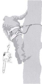
Attach the tree trimming chainsaw to the rear center point of the harness.
