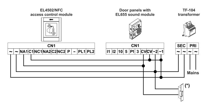
(\*) Lock releases connected to audio door entry systems with 4+"n" installation operate at 12Vac: fit the varistor supplied with the access control module directly to the lock release terminals.
