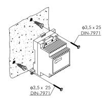
Install the transformer in a dry and protected location.
