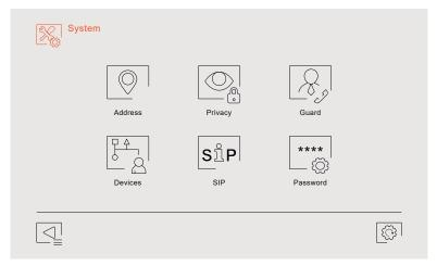
To re-set the monitor settings to a factory values, we must press over the icon with the bottom right on the screen. The following screen will appear and we must confirm the factory reset of the monitor settings.
