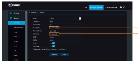
The IP address of the camera should be modified with a value between 10.128. XX.XX to 10.254.XX.XX
