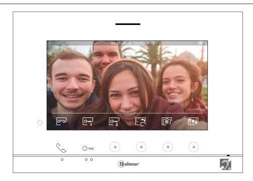
This screen is displayed during a communication process. In the top centre of the screen, the date and time are shown and, on the right, the source of the image is displayed (door panel 1 to door panel 4, camera 1 to camera 4).
