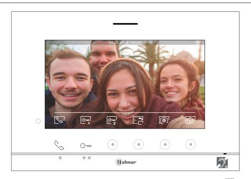
This screen is displayed when you receive a call or when you press the button below icon During a call, icon displayed on the screen will blink green (during the call process). In the top centre of the screen, the date and time are shown and, on the right, the source of the image is displayed (door panel 1 to door panel 4, camera 1 to camera 4). The call has a duration of 45 seconds.
