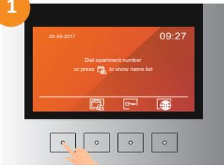
1 Access to the configuration by pressing 5 times in the indicated pushbutton.
