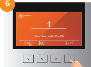
6 Enter, through the keypad, the block number "1" and press over the validate option.
