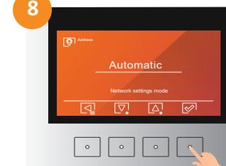
8 Choose the automatic IP assignment. In this way, the door panel will take the **192.168.100.101** IP address. The IP address will be different if other parameters were entered.
