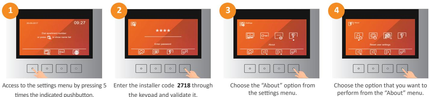
If you choose any settings reset, the door panel will show a confirmation screen to avoid accidental settings reset. Confirm the reset in this screen and wait until the panel is operative again.
