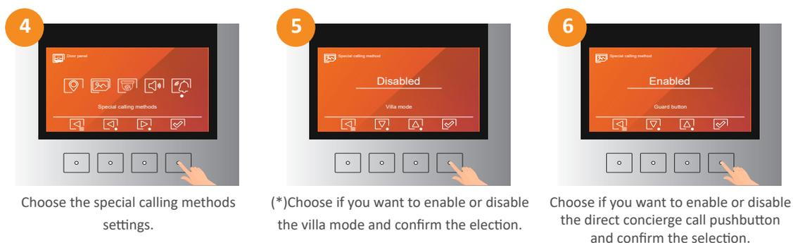
(\*)In villa mode the door panel makes a call to the address number 1 with only pressing the bell icon push button.
