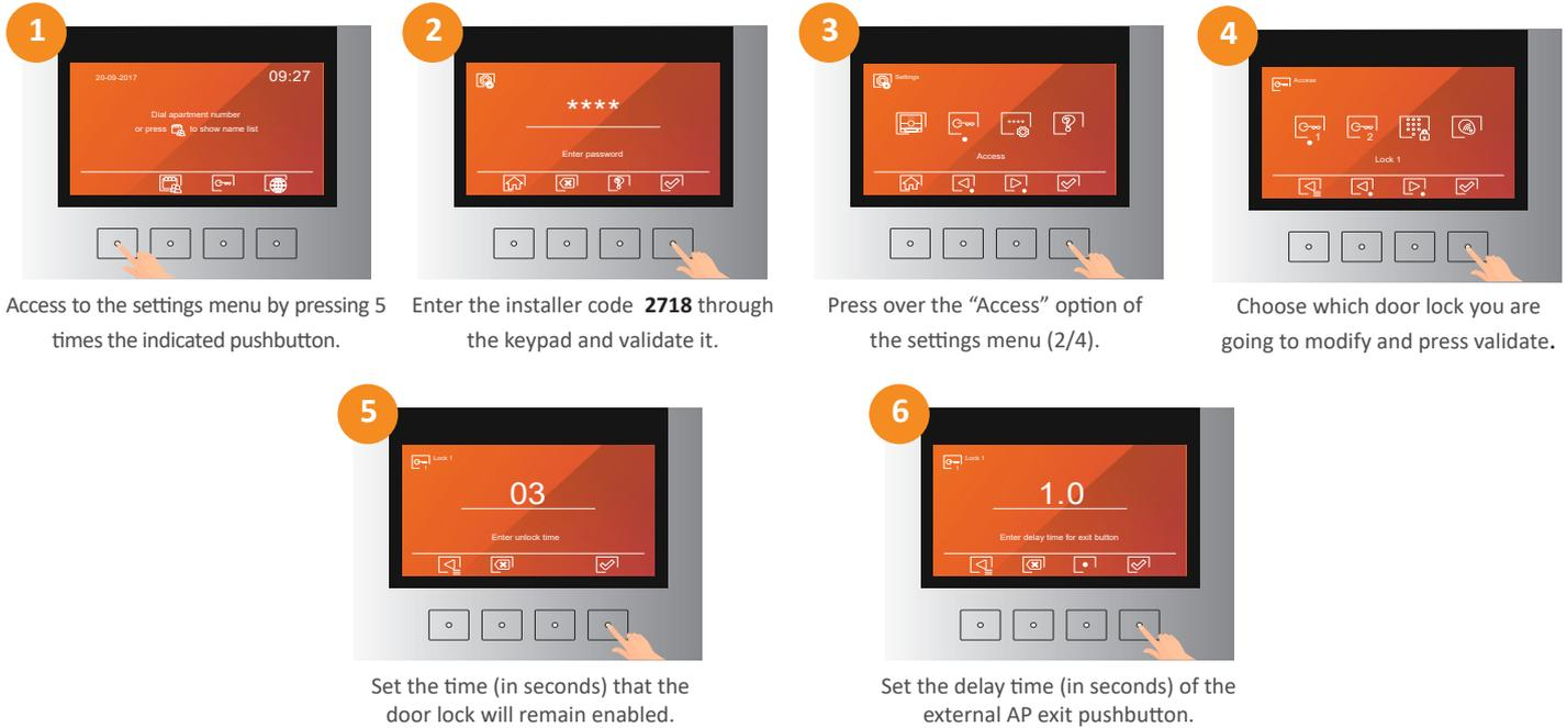
You must do the same procedure to modify the door lock 2 parameters. Only, you must choose the “Lock 2” option in the step 4.
