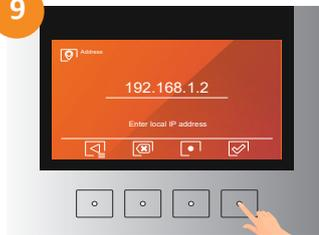
9 Enter the desired IP address for the door panel and press validate.
