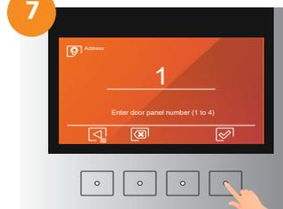
7 Enter through the numeric keypad the **panel number "1"** and press validate. Contact with the Golmar technical service to install more than 4 door panels.
