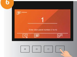
6 (\*\*)Enter through the numerical keypad the number of **general panel** and press validate
