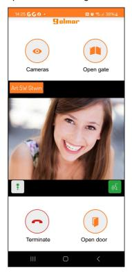
Press the "Camera" button to go to the next door panels or to any connected surveillance cameras. Press the "Open door" button to open the entrance door and press the "Open gate" button to open the driveway gate.
