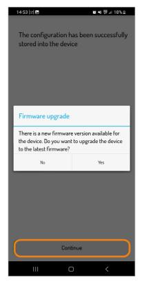
19. By pressing the "YES" button you can update the firmware of the device, skip to point 7 in chapter "Updating the firmware" on page 15.Pressing the "No" button closes the screen without updating the device.
