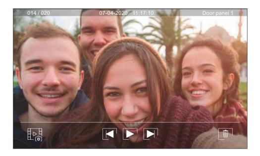
To view a video recording, select it in the list. The recording will be displayed full screen. Use the scroll arrows to display the next or previous recording. From this screen, you can also delete the recordings individually, which always requires your confirmation. Use icon to start playback of the video selected; press icon to stop video playback.
