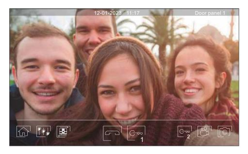
This screen is displayed during a communication process. In the top centre of the screen, the date and time are shown and, on the right, the source of the image is displayed.
