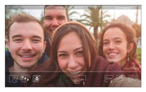
This screen is displayed when receiving a call or pressing icon of the main menu. During a call, icon displayed on the screen will blink green (during the call process). In the top centre of the screen, the date and time are shown and, on the right, the source of the image is displayed. The call has a duration of 45 seconds.
