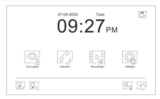
If the device is in standby (screen off), touch any part of the screen to activate it and bring up the main menu. The device will return to standby mode after 20 seconds without activity.
