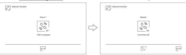
To perform an internal broadcast process, select the monitor to establish communication and then press icon (; it is now possible to talk, listen, and raise and lower the communication volume from each of these 2 monitors. Communication will last for 90 seconds or until icon [] is pressed.
