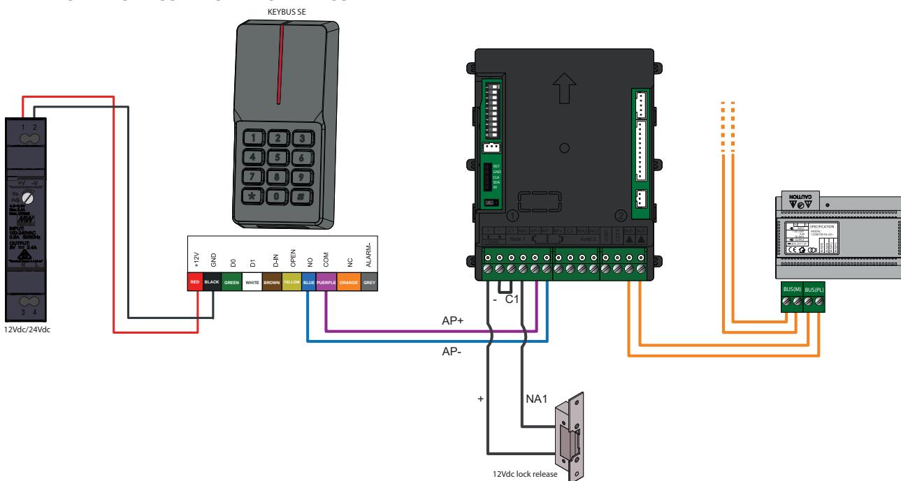
NOTE: The intercom AP (door opener) does not activate the door opener until the KeyBus SE reader pulse is completed. To avoid opening delays, set the minimum pulse on the reader (1 second):
