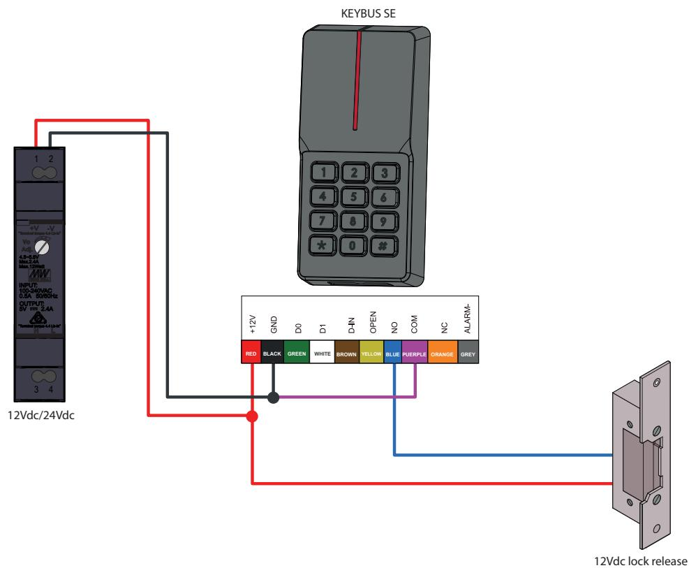
By default, the reader is set up to operate in standalone mode.
