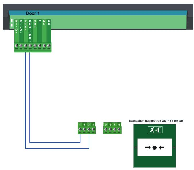
\*In case to connect the evacuation push button to the output push button terminal of the controller to re-securize the door(s), the push button will need to be re-armed and the door(s) will need to be manually secured in iP Opener Manager.
