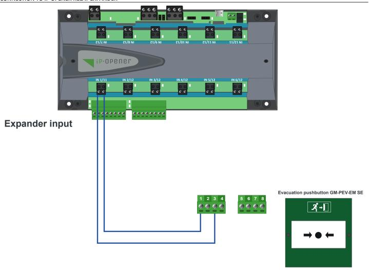
\*In case to connect the evacuation push button to the input expander, the system can be configured so that the door or doors will be secured again after arming the push button again.
