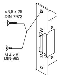
**IMPORTANT:** The lock release must be Golmar 12V AC or DC.
