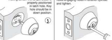
B. Press interior assembly flush against door making certain the torque blade is properly positioned in latch hole. Key hole should be in down position.
