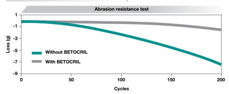
Taber abrasion resistance test on H20 concrete and on H20 concrete with 2 layers of 100 g/m² of Betocril.
