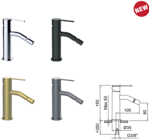
Bidé monomando con aireador a rótula y flexibles 3/8" >350mm. Single-lever bidet mixer with swivel aerator and flexible hoses 3/8" >350mm.
