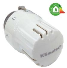
The thermostatic W6 allows an individual adjustment of the ambient temperature. They are proportional and permanent regulators. These heads react automatic to the variation of the room temperature. If the temperature increases, for example, as an effect of the solar radiation, the liquid sensor limits the water circulation in the heater, reducing the pass of the valve.
