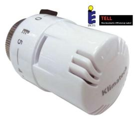
The thermostatic W6 allows an individual adjustment of the ambient temperature. They are proportional and permanent regulators. These heads react automatic to the variation of the room temperature. If the temperature increases, for example, as an effect of the solar radiation, the liquid sensor limits the water circulation in the heater, reducing the pass of the valve.
