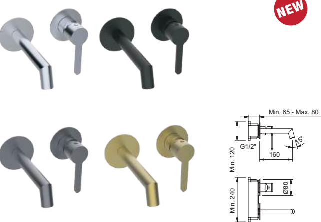
Lavabo empotrar 1/2" con aireador. Concealed basin mixer 1/2" with aerator.
