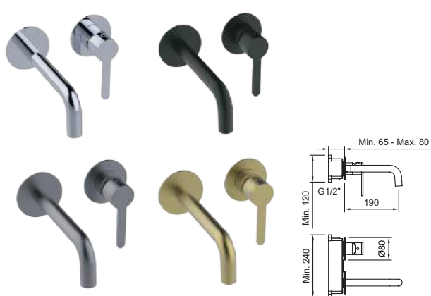
Lavatório de embutir 1/2" com areador. Concealed basin mixer 1/2" with aerator.
