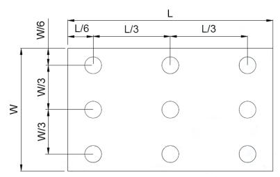
Bmax : The measured maximum luminance of all measurement position.
