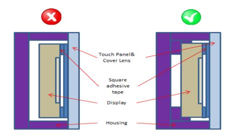
(3) TP needs to work in environment with stable stray capacitance. In order to minimize the variation in stray capacitance, all conductive mechanical parts must not be floating. Intermittent floating any conductive part around the touch sensor may cause significant stray capacitance change and abnormal touch function. It is recommended to keep all conductive parts having same electrical potential as the GND of the touch controller module.
