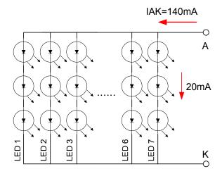
Note(6) When LCM is operated over 60°C ambient temperature, the IAK of the LED backlight should be adjusted to 105mA max
