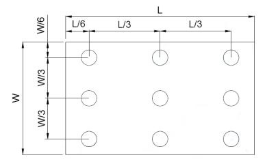
Bmax: The measured maximum luminance of all measurement position.
