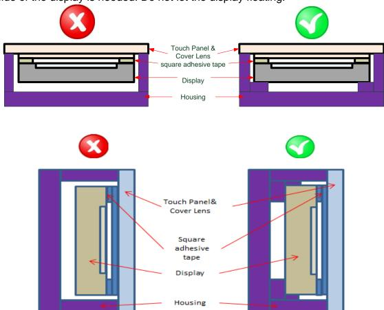
3) TP needs to work in environment with stable stray capacitance. In order to minimize the variation in stray capacitance, all conductive mechanical parts must not be floating. Intermittent floating any conductive part around the touch sensor may cause significant stray capacitance change and abnormal touch function. It is recommended to keep all conductive parts having same electrical potential as the GND of the touch controller module.
