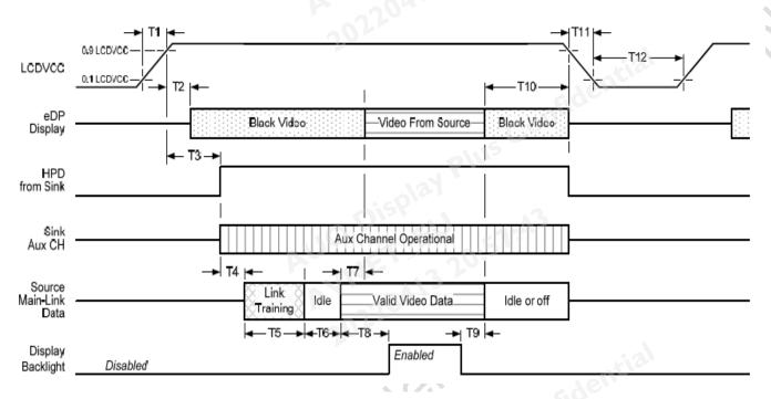
Display port interface power up/down sequence, normal system operation
