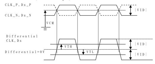
$\begin{array}{l} CLK\_P,\, CLK\_N \\ Dx\_P,\, Dx\_N \quad x = 0,1,2,3 \\ |VID| = |**\_P-**\_N| \\ VCM = (**\_P+**\_N)/2 \\ P: +,\, N: - \\ **:\, CLK \text{ or } Dx \end{array}$
