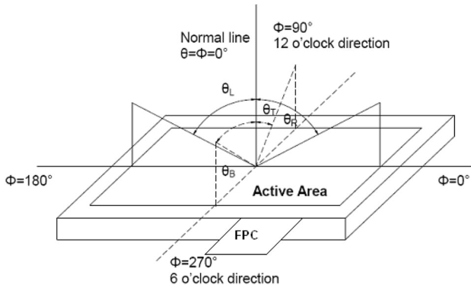
**Fig2. Definition viewing angle**
