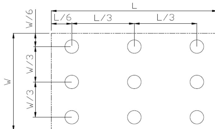
**Fig5. Luminance Uniformity Measurement Locations(9 points)**
