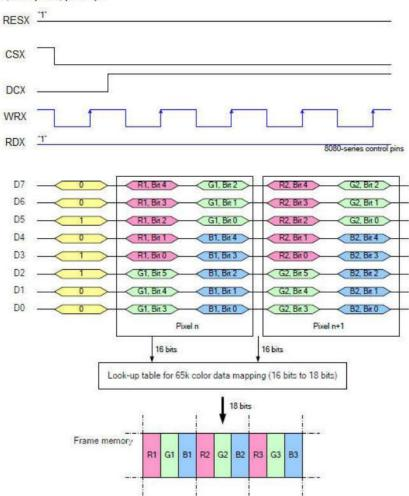
Note 1: The data order is as follows, MSB=D15, LSB=D0 and picture data is MSB=Bit 5, LSB=Bit 0 for Green, and MSB=Bit 4, LSB=Bit 0 for Red and Blue data.
