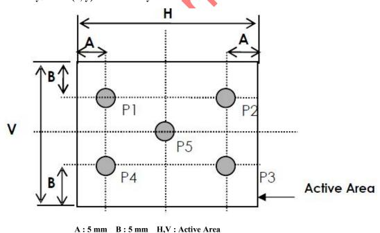
Light spot size A=7mm, 500mm distance from the LCD surface to detector lens
