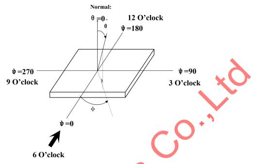
Note 7. Surface luminance is the LCD surface from the surface with all pixels displaying white. Refer to figure as below.
