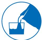
Add approx 11.5 litres of clean water per 25kg bag to mixing bucket. Gradually add the plaster to water whilst mixing
