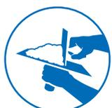
Complete 2<sup>nd</sup> coat, the total thickness for both coats should be a minimum of 2mm
