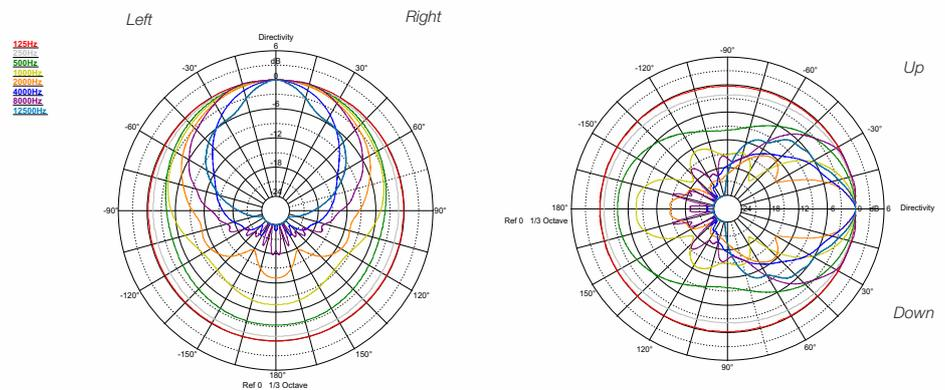
NOTES: Frequency response measured at 4m (13,12ft). For better detail, only light smoothing (1/12th octave) has been used. Polars were acquired by placing the unit on a computer controlled turntable inside a 300 m<sup>3</sup> (10594 ft<sup>3</sup>) anechoic chamber. Measurement distance is 4m (13,12ft).
