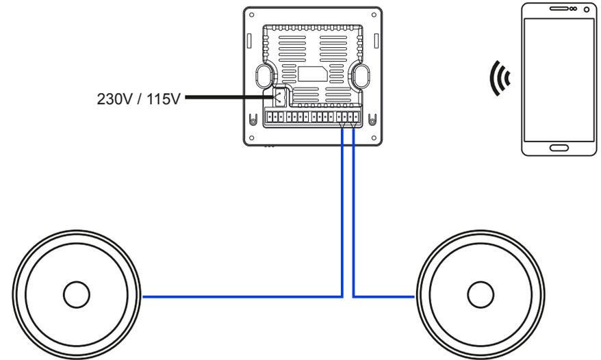
4ohm load per channel, BT audio input from a tablet or mobile phone
