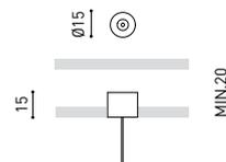
Wire Trimless Accessory is a collection of accessories for fitting tensioners and cables to Arkoslight luminaires suspended directly from the ceiling with any visible ceiling rose or fixings. This achieves a minimalist application with a visually tidy finish.
