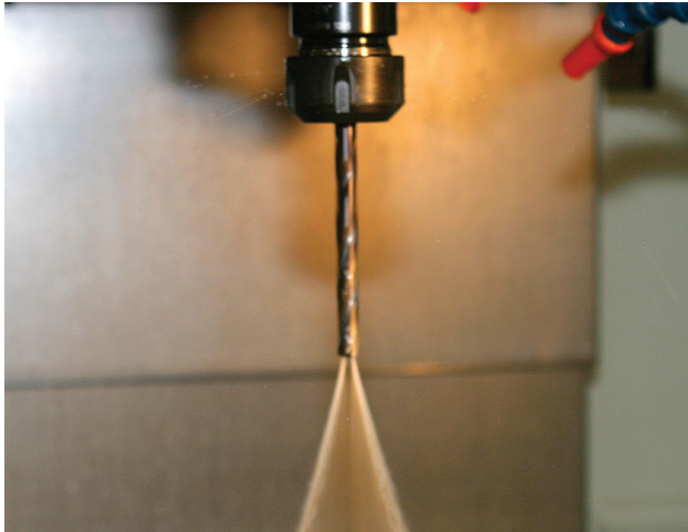
Use ER Coolant Rings with o-ring for coolant-thru cutting tools.
