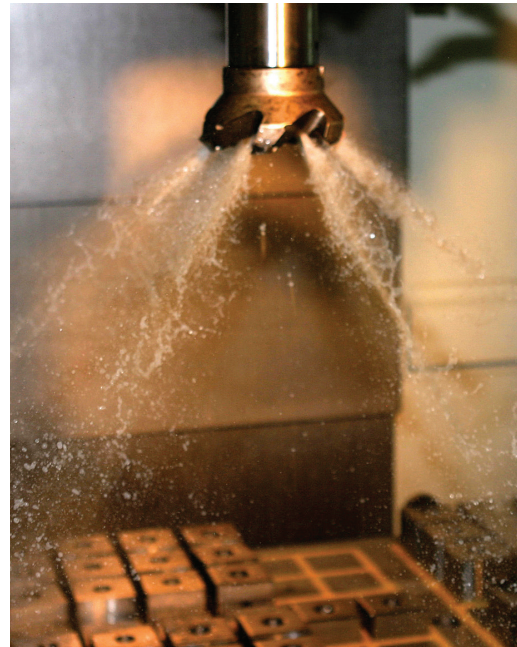
CoolBLAST arbor screw provides coolant path.
